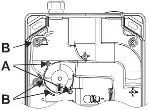
Fig. 46 Removing the aspirating fan unit
