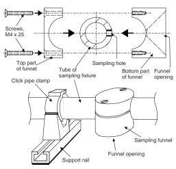
Fig. 27 Using sampling funnels
