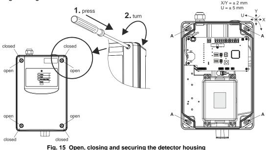
rig. to open, closing and securing the detector housing
