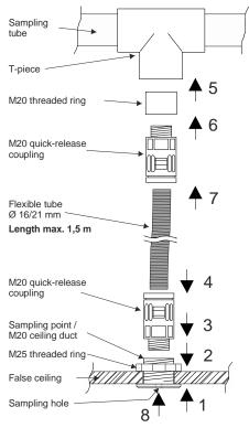
Fig. 28 Mounting the ceiling bushing
