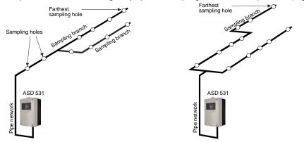
Fig. 7 Examples of planning with "ASD PipeFlow" calculation
