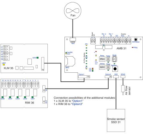
Fig. 2 Block diagram
