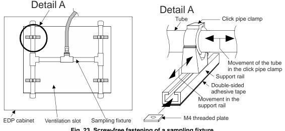
Fig. 23 Screw-free fastening of a sampling fixture
