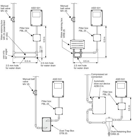
Fig. 29 Mounting accessory parts
