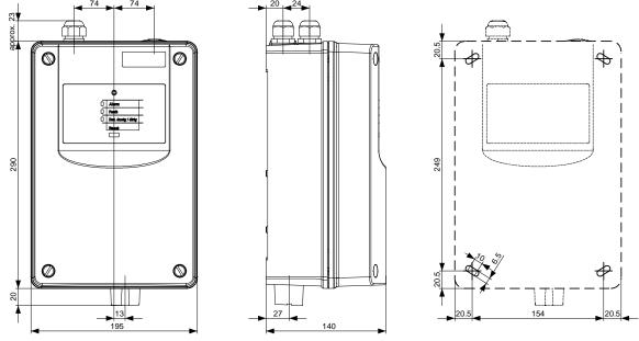
Fig. 14 Detector housing dimensioned drawing and drilling plan
