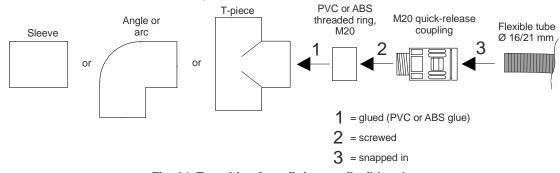
Fig. 24 Transition from fittings to flexible tube
