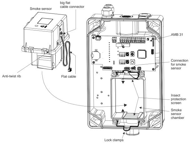
Fig. 30 Deploying the smoke sensors
