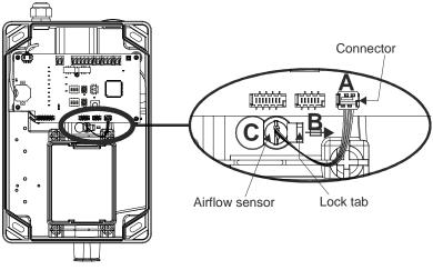
Fig. 47 Removing the air flow sensors
