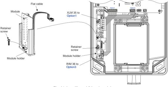
Fig. 31 Installing additional modules
