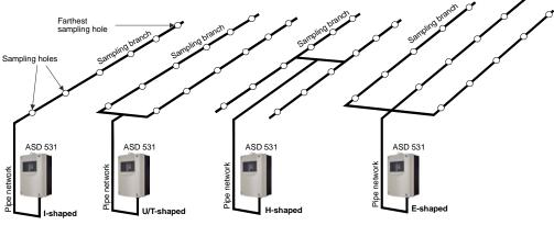
Fig. 8 Examples of planning without "ASD PipeFlow" calculation
