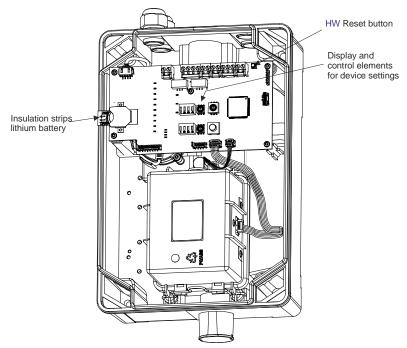
Fig. 40 Detector housing opened for commissioning
