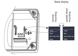
Fig. 18 Turning the labelling strips
