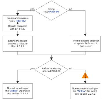
Fig. 13 Workflow for project-specific programming and adjustment
