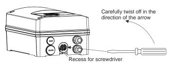
Fig. 17 Removing the air outlet pipe plug
