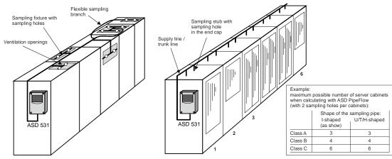
Fig. 11 Equipment monitoring layout variants (examples)
