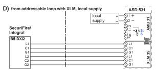
Fig. 35 Control via the "Reset external" input
