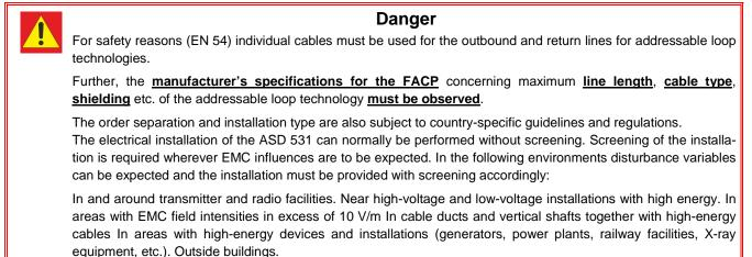
If screening is used, the cable screening in the ASD 531 is to be connected to an additional support terminal. The cable screening must **not** be connected to the minus or ground terminal of the AMB 31.
