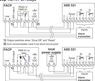
Fig. 37 Connection on selective identification or addressable loop
