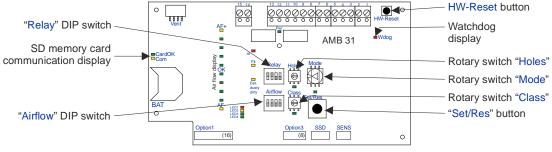
Fig. 41 Control and indicator elements on the AMB 31
