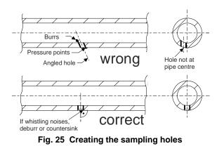
For equipment monitoring, the sampling holes are drilled in the sampling fixture. The sampling holes are drilled into the sampling fixture in the direction of the air outlet from the object to be monitored. If required, these sampling holes can be fitted with sampling funnels (Sec. 5.5.10).
