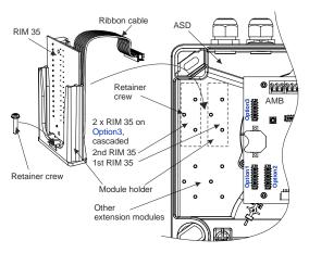
Fig. 2 Installing the RIM 35
