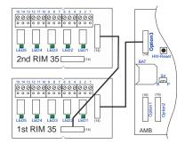
Fig. 3 Wiring the RIM 35
