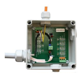
Connection unit for one or two temperature sensor cable SEC15 including an universal connection module UCM.
