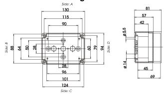
Fig. 3 Dimensioned drawing (in mm)
