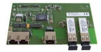
Fig. 22 B6-NET2-FXS network unit
